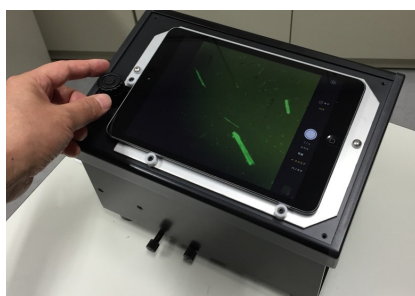
Detection system for airborne asbestos release in environment
